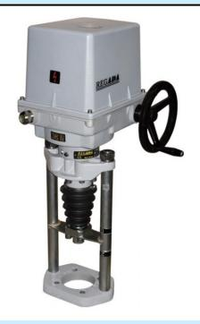
492 Type number: Switching-off thrust: 9000 to 25000 [N] [mm/ Operating speed: 10 to 120 min] Operating stroke: 8 to 100 [mm] Ambient temperature: -25 (-50) to +55 [°C] Protection enclosure: IP 65, IP 67 Operating position: any position Weight: 17 to 21,5 [kg]
