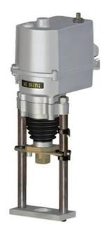
Type number: 472 Switching-off thrust: 250 to 1100 [N] [mm/ Operating speed: 5 to 40 min] Operating stroke: 6 to 25 [mm] Ambient temperature: -25 to +55 [°C] Protection enclosure: **IP 67** Operating position: any position Weight: 3,3 to 3,7 [kg]
