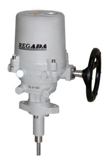
Type number: 535 Switching-off thrust: 1400 to 6900 [N] [mm/ Operating speed: 10 to 80 min] Operating stroke: 4 to 40 [mm] Ambient temperature: -25 to +55 [°C] Protection enclosure: **IP 67** Operating position: any position Weight: 6,5 to 8,5 [kg]
