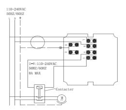
Wiring diagram for connecting three-phase 380 V pumps through a contactor switching. (Specifications for main contactor: Minimum capacity of 4 kW or contact approx 5.5 Hp, 230 V).
