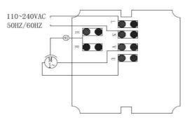
Wiring diagram to connect 230 V single-phase pumps over 1.1 kW (1,5 HP) through a contactor switching. (Specifications for main contactor: Minimum capacity of 4 kW or contact approx 5.5 Hp, 230 V).
